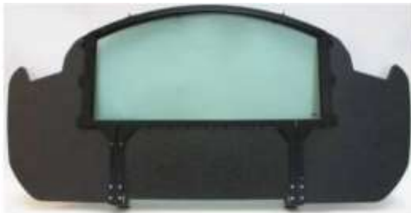
Figure 5. Front panel with bulletproof glass [3]
