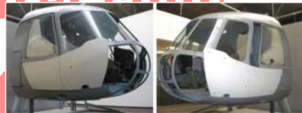
Figure 4. Outside ceramic composite panels installed [3]
