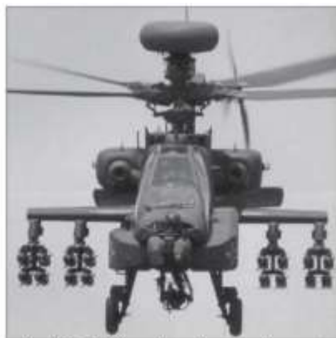
Figure 1: McDonnell Douglas AH-64D Longbow Apache demonstrator is seen carrying a full weapons load of 16 Hellfire missiles during a pres demonstration in the mid 1990s. By 1997 this helicopter was wearing Boeing titling [2]
