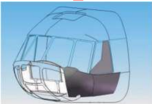
Figure 2. Outside ceramic composite panels [3]
