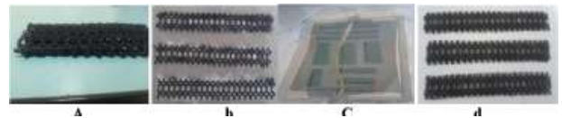
Figure 2: a) 3D fabric b) chicken feather fiber between 3D fabrics layers c) prepared sandwich under vacuum infusion d) specimens after vacuum.
